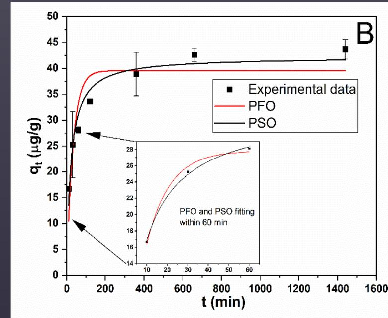
(A) Adsorption kinetics of DMSO<sub>2</sub> onto [Emim]NTf<sub>2</sub> coated biochar, (B) Pseudo first order (PFO) and Pseudo second order (PSO) kinetics
